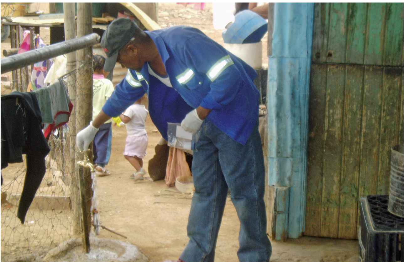
Saul Maans, of Middelpos in the Northern Cape, using an H 2 S testkit to take a water sample. Saul tested water samples using the H 2 S kit as part of the Aquatest 2 Project, and then sent the results using the WQR (Water Quality Reporter) application, which was uploaded on his cellphone.
